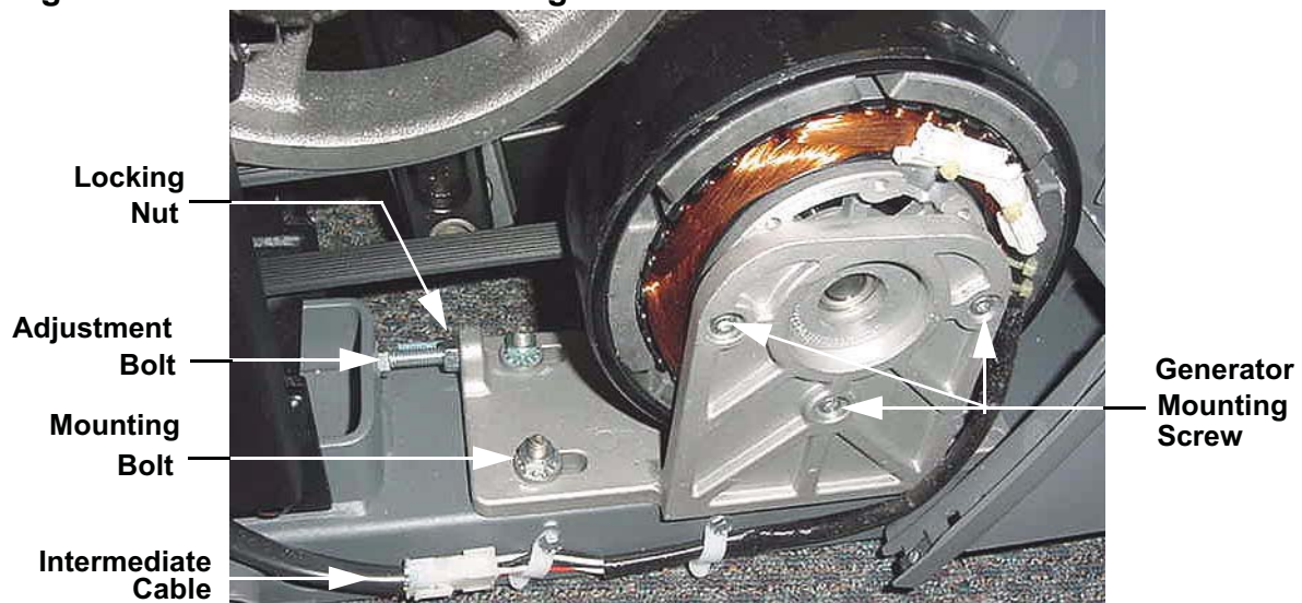
Diagram 7.19 - Generator Mounting
